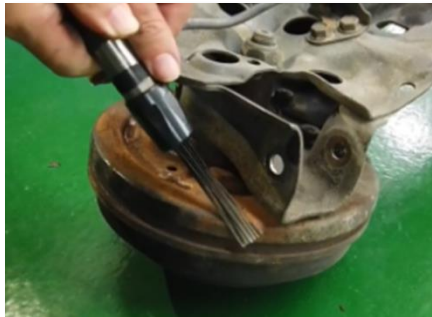
Clear away rust, debris with bigger area
