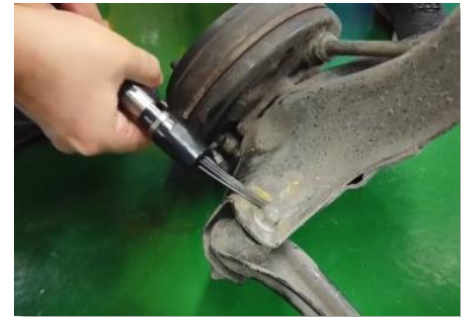
Remove rust and dirt on bolt before breakaway
